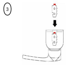
The tumblers are shaped to fit into the slots
