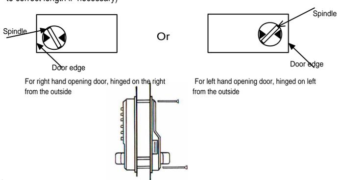
BEFORE CLOSING THE DOOR check the operation of your lock front & back\*
